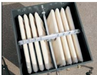
Bag filters made of cotton (standard) with mechanical shaker mechanism
