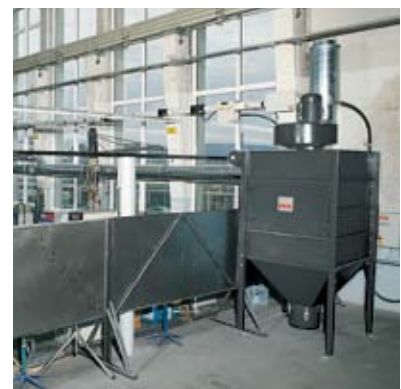
Modular extractor DUSTEX in a metalworking application
