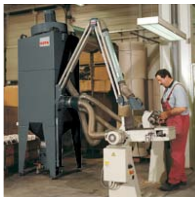
Wet separator NA-K extracting aluminum dust
