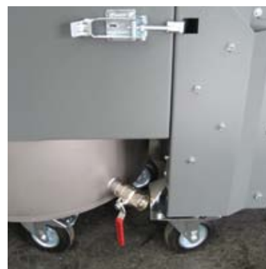
Valve for draining contaminated water
