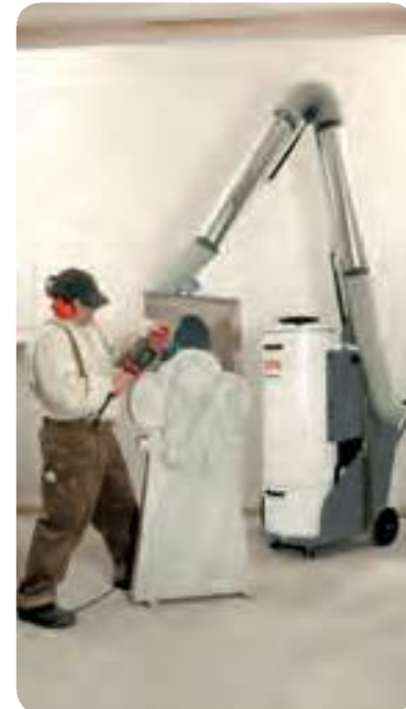
DUSTOMAT-16 M – direct extraction of fine stone dust
