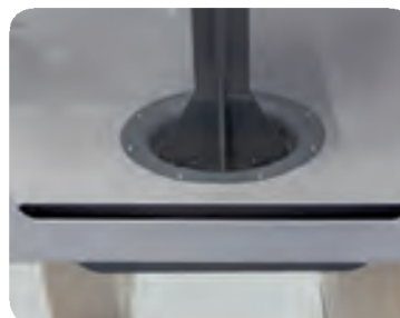
Suction nozzle in front area
