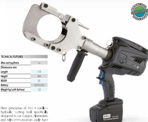
hydraulic cutting tool specifically ing a max overall diameter of 95 mm. The blades are manufactured from high strength special Steel, heat treated to ensure a long service life. New Li-lon 18 V 4 Ah batteries offer a higher capacity than 14.4 V 3 Ah, while greater cutting speed and cutting force result from a revitalised hydraulic system with double speed action.
