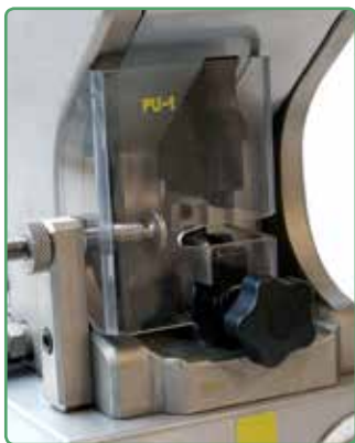
PNB-1 detail of the crimping zone with PU-1 guard.
