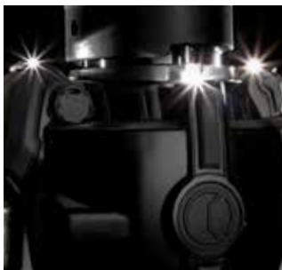
4 LED lighting of the working area
