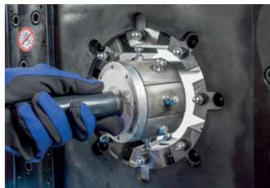
Die sets can be installed into the master dies with a QuickChange-tool one set at a time.
