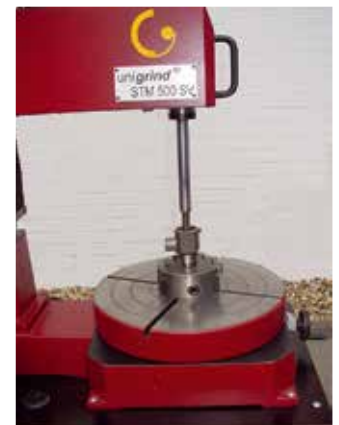
Grinding safety relief valve on rotary table
