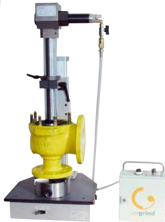
SVS 1 grinding a valve on machine stand
