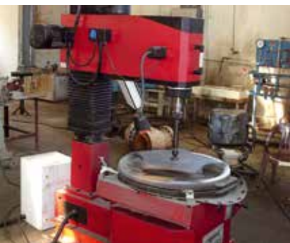
STM 800 E Grinding of gate valve wedge
