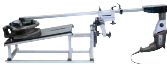
SLIM 300 grinding of gate valve wedge
