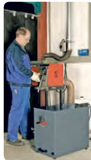
Mini dust collector TK connected to a deburring machine
